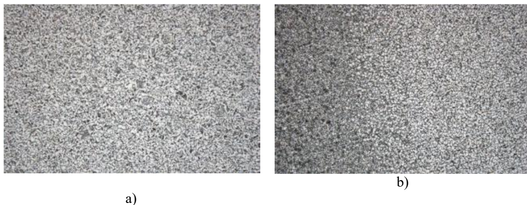
Figure 11. Microstructure of gland seal water pipe. Base metal (a), Across heat affected zone (boxed area “c”), 200x magnification (b)
